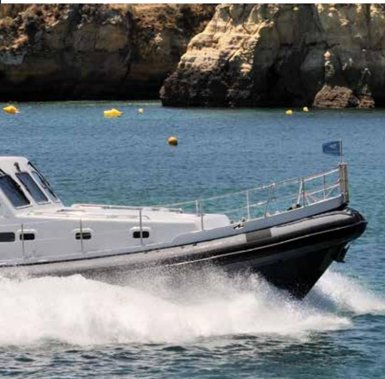
Holding 1,300 gallons of fuel and 260 gallons of water, the No Limit 1640 has an extensive range at lower speeds. At 8 knots, she burns 4.4 gph and, at the time of writing, the 50-footer, Four Seasons, was crossing the Atlantic, following the northern route via Iceland and Greenland. With a draft of four feet and an air draft that can be reduced to 12 feet by lowering the radar arch, this No Limit is equally adept at cruising inland waterways.
